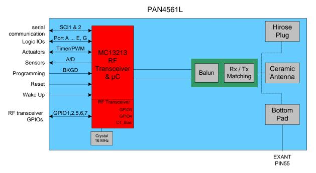
The MC13213 is used in single port configuration with its internal Tx/Rx switch. For more details refer to chapter 7.1.
